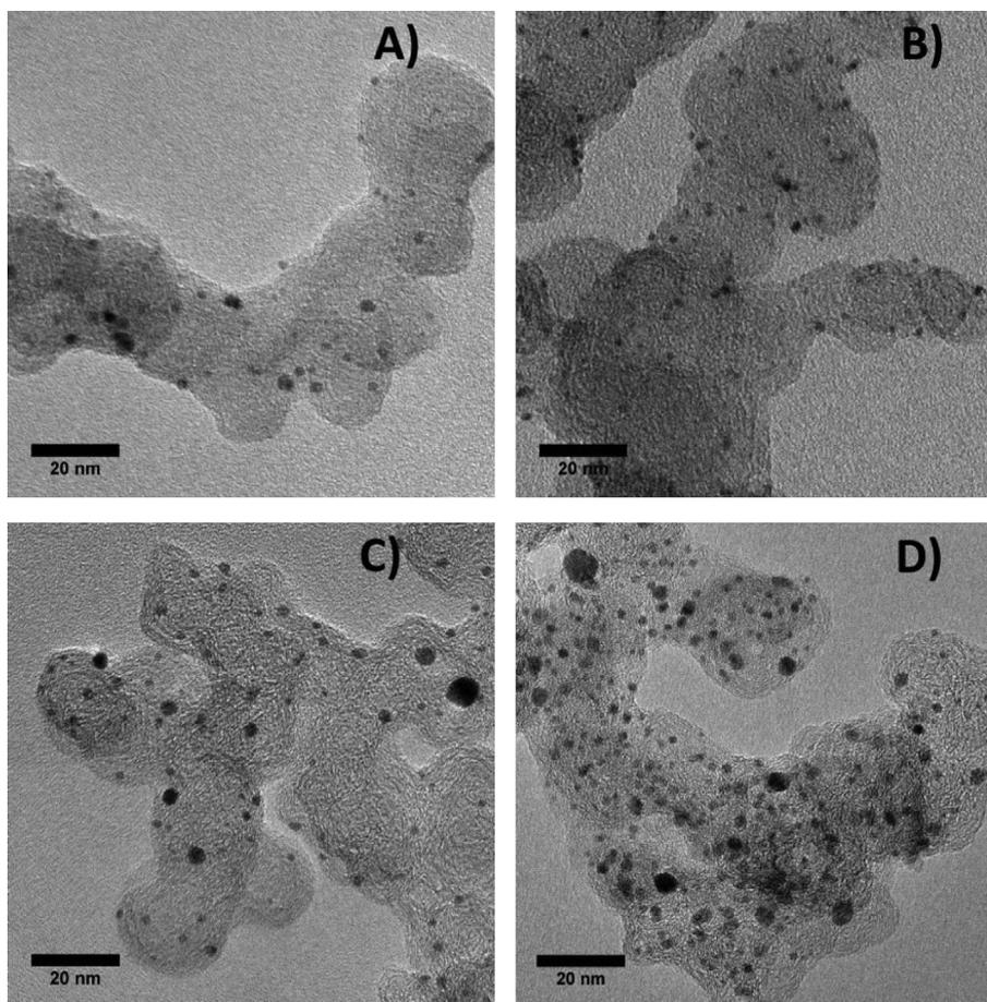
Fig. 1. TEM micrographs of  $Pt_xCo_{1-x}/C$  catalysts. A) Leached/PtCo/C(I), B) leached/PtCo/C(II), C) leached/HT PtCo/C(I), and D) leached/HT PtCo/C(II).
