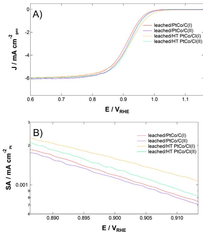
**Fig. 4.** A) Representative ORR polarization curves of the  $\text{Pt}_x\text{Co}_{1-x}/\text{C}$  catalysts recorded in positive going scan rate of  $50 \text{ mV s}^{-1}$  in oxygen saturated  $0.1 \text{ M HClO}_4$  electrolyte; Rotation rate was  $1600 \text{ rpm}$ ; B) corresponding Tafel plots of the specific activity for the ORR.
