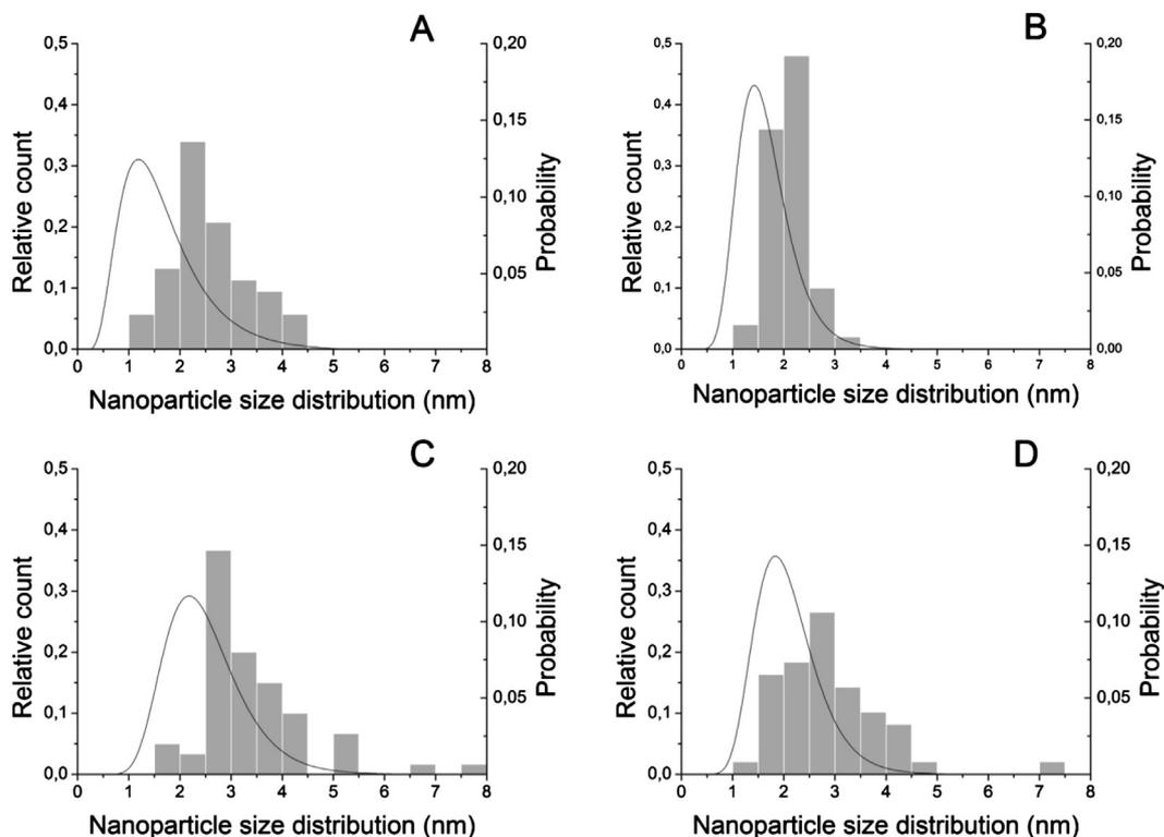
**Fig. 2.** Particle size distributions of carbon supported  $Pt_xCo_{1-x}$  NPs established from TEM (left scale) together with the particle size distribution obtained by SAXS. An estimate of the average particle size (diameter) is given in the brackets in nm (TEM/SAXS). A) Leached/PtCo/C(I) ( $\sim 2.8/1.5$ ), B) leached/PtCo/C(II) ( $\sim 2.0/1.6$ ), C) leached/HT PtCo/C(I) ( $\sim 3.4/2.4$ ) and D) leached/HT PtCo/C(II) ( $\sim 2.74/2.0$ ).
